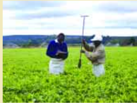
> In field soil sampling to monitor changes in organic matter and nutrient levels
